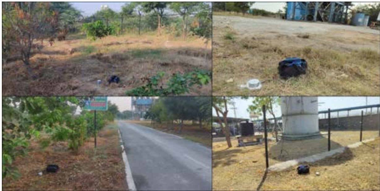
Photograph 1. Monitoring of blast induced ground vibration at different locations in the periphery of Kayad UG mine.
